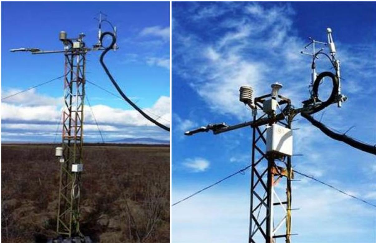
**Figure 3** – Eddy-covariance towers at the Chersky research site (Photograph: Göckede). The system consists of a heated sonic anemometer (METEK USA1), an open-path gas analyzer for CO<sub>2</sub>/H<sub>2</sub>O (LiCor 7500, only right picture), and the inlet line for a closed-path gas analyzer for CH<sub>4</sub>/CO<sub>2</sub>/H<sub>2</sub>O (Los Gatos FGGA).
