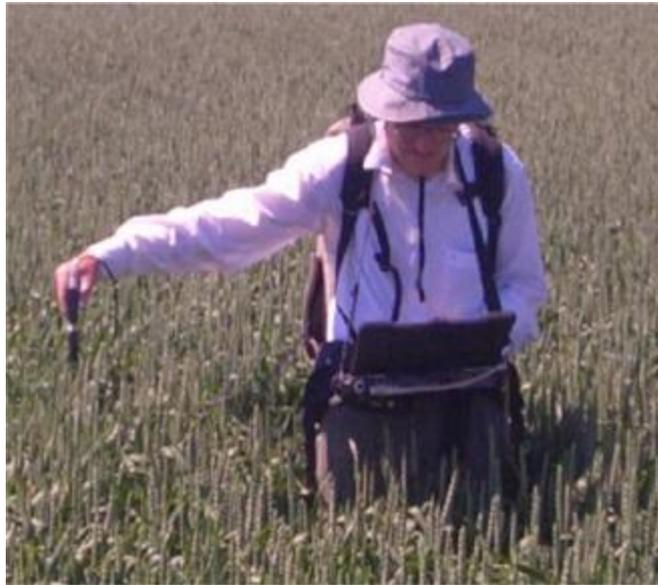
**Figure 1:** Measuring hyper spectral data of a cereal field using a field spectrometer
