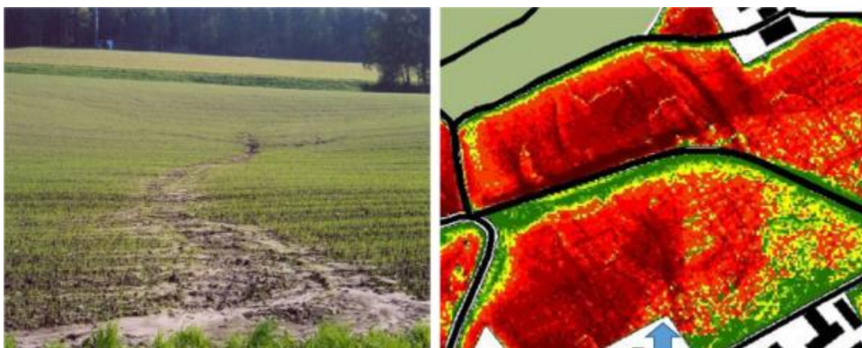
Figure 2 – Comparison of mapped and photographed erosion damage with modelled erosion risk. The erosion in the thalweg is well represented by the model.
